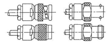
Insert the cable as far as possible in the plug or socket connection and tighten the pressure screw.
