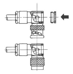
Insert the cable as far as possible in the plug connection and tighten the pressure screw. Tin plating the inner conductor with the contact pin. Remove excess solder. Tightly screw the locking screw.
