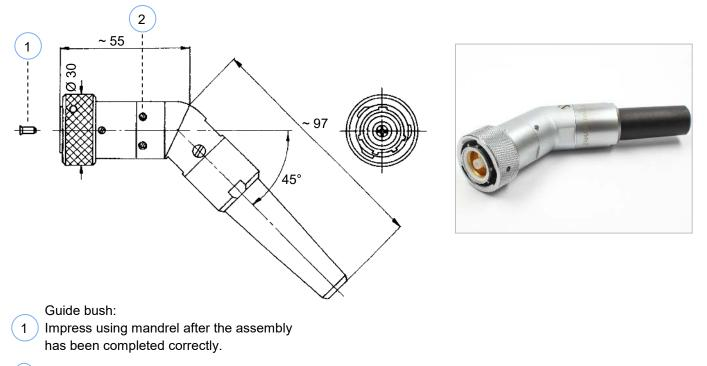
Cable outlet can be adjusted radially in 30° steps in all directions
