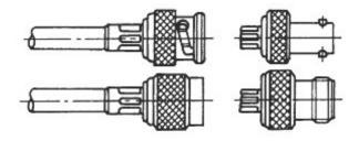
Place the plug or socket with the cable in the crimping pliers so that the plug or socket body is positioned at the press-in indentation, than crimp.
