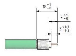
Strip the insulation from the cable.
