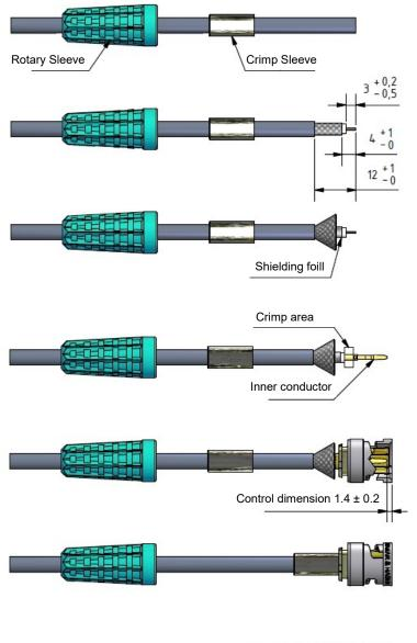
Slide the Rotary Sleeve and the Crimp Sleeve over the cable.
