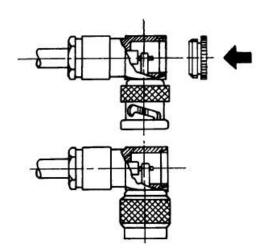
Insert the cable as far as possible in the plug connection and tighten the pressure screw.
