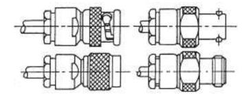
Insert the cable as far as possible in the plug or socket connection and tighten the pressure screw.
