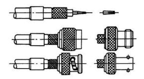
Slide the contact pin or contact socket as far as the dielectric on the inner conductor and crimp, using the crimping pliers.
