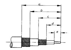
Strip the insulation from the cable as specified in the table.
