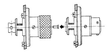
Fix panel cable plug/panel cable socket onto the mounting panel.
