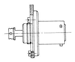
Fix the panel cable plug onto the mounting panel.
