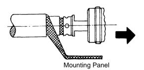
Insert the cable in the plug-in connection. Finally, solder the inner conductor and the inner shield.
