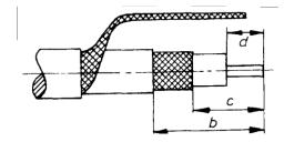
Strip the insulation from the cable as specified in the table.
