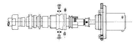
Fix the panel cable plug onto the mounting panel.
