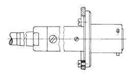
Insert the cable in the plug-in connection. Then solder the inner conductor and the inner shield. Slide forward the outer sleeve, screw tight and fasten using two threaded pins.
