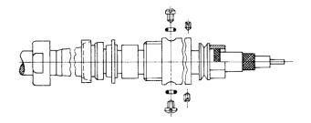
Slide the cable clamp and fittings over the cable. Place the outer braiding around the tension relief ring, slide over the large clamping sleeve, and solder or crimp using the crimping pliers. (For soldering, no clamping sleeve is required.)
