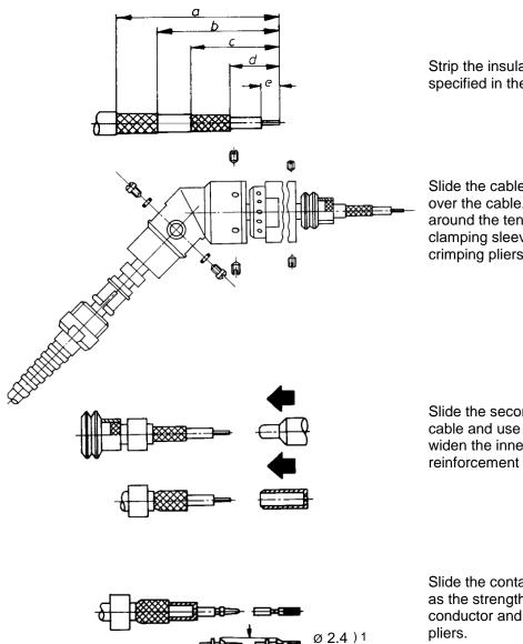
Strip the insulation from the cable as specified in the table.
