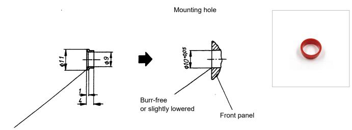
Coding ring pressed into mounting hole
